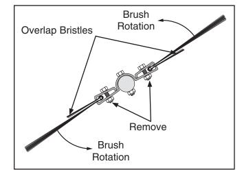
Figure 15. Brush assembly (end view).
